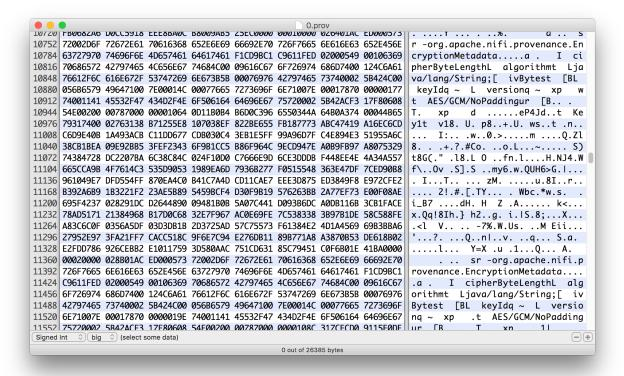
On record read, the process is reversed. The encryption metadata is parsed and used to decrypt the serialized bytes, which are then describilized into a ProvenanceEventRecord object. The delegation to the normal schema record writer/reader allows for "random-access" (i.e. immediate seek without decryption of unnecessary records).
