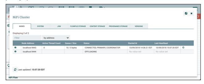
Nodes that remain in "Offloading" state due to errors encountered (out of memory, no network connection, etc.) can be reconnected to the cluster by restarting NiFi on the node. Offloaded nodes can be either reconnected to the cluster (by selecting Connect or restarting NiFi on the node) or deleted from the cluster.
